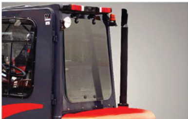
Upward Exhaust Pipe I
